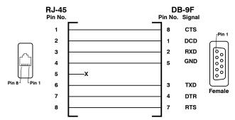
Figure 4.1: DX9F-DTE-RJ Snap Adapter Interface
